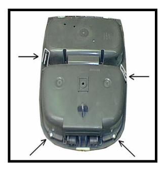
3. Attach four (4) pod mounting brackets (item 14 pg 2) to front and rear of bezel with four (4) 6-32 X 1/2" screws (item 4 pg 2) and four (4) 8-32 KEPS nuts (item 1 pg 2). See Figure 10.
